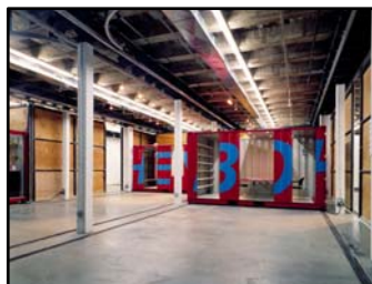
CREATING FLEXIBILITY SHIPPING CONTAINERS HOUSING OFFICE FUNCTIONS MOVE ON TRACKS TO CHANGE THE SPACE FOR MULTIPLE USES
