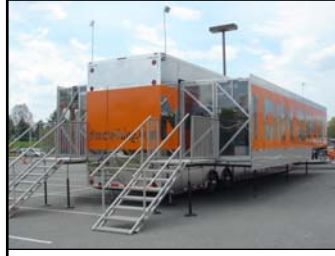
TRIPLING SPACE A 53 FOOT LONG TRUCK TRIPLES IN SIZE AND OPENS WITH THE PUSH OF A BUTTON TO BOTH SIDES.
